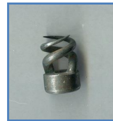
Civil War .58 cal. "Bullet Worm" Extractor/Wiper - Model 1861 Found at Gettysburg
